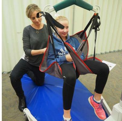
Attach to hoist. Please note the position of the hoist, the base is open. Check bottom is supported by sling
